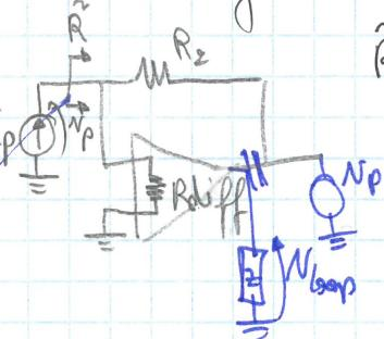
$$\tilde{R}^* = R_{diff} // R_2, \text{ calcolo } G_{loop}^* = -\frac{R_{diff} \cdot A_0}{R_{diff} + R_2}$$
