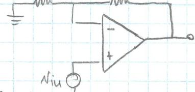
$$G_{loop}(s) = \frac{-R_1}{R_1 + R_2} \cdot \frac{A_0}{(1+sT_1)(1+sT_2)} = \frac{-10^2}{10^2 + 10^5} \cdot \frac{10^6}{(1+sT_1)(1+sT_2)} = \frac{-10^4}{(-)(-)}$$
