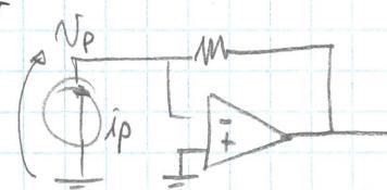
~~Se avessi Rdiff~~ Calcolo  $R_{in}$ :  $G_{loop} = -\frac{R_{diff}}{R_{diff} + R_f} \cdot A_o$
