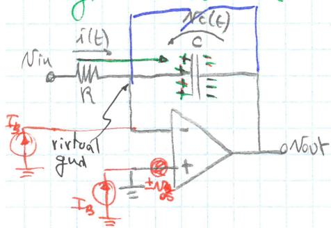
$$i(t) = \frac{V_{in}(t)}{R} \quad Q(t) = \int_0^t i(\tau) d\tau$$
