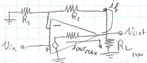
$$i_{out}|_{MAX} = i_{R_L} + i_f = \frac{V_{out}|_{MAX}}{R_L|_{MIN}} + \frac{V_{out}|_{MAX}}{R_L + R_e}$$
