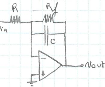
$$T(s) = -\frac{R_f}{R} \frac{1}{1+sR_f C} \quad \text{per la DC } G = -\frac{R_f}{R}$$
