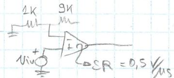
$$\text{Nei datasheet } V_{out} = A_{out} \sin \omega t \quad \frac{dV_{out}}{dt}|_{MAX} = A_{out} \cdot \omega \cos \omega t|_{MAX} = A_{out} \cdot \omega = A_{out} \cdot 2\pi f$$
