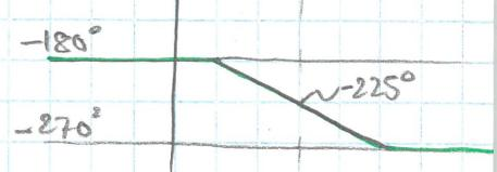
$$\angle T(j\omega) = \begin{cases} \omega \ll R_2 C_2 & = -180^\circ \\ \omega = R_2 C_2 & = \pi - \frac{\pi}{4} = 45^\circ + 180^\circ = 225^\circ \\ \omega \gg R_2 C_2 & = \pi - \frac{\pi}{2} = 180^\circ - 90^\circ = 270^\circ \end{cases}$$
