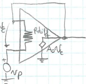
$$R_{in} = \frac{N_p}{i_p} \quad i_p = \frac{N_e}{R_{diff}} = \frac{N_p - A_0 N_e}{R_{diff}} \quad N_e = N_p - A_0 N_e \quad N_e = \frac{N_p}{1 + A_0}$$
