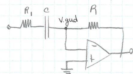
$$z_1 = R_1 + \frac{1}{SC} \quad z_2 = R \quad T(s) = \frac{-SCR}{1+SCR_1}$$
