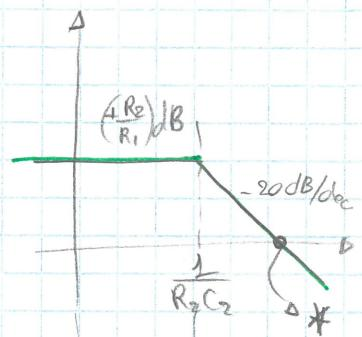
$$\angle T(j\omega) = -180^\circ - \arctg(R_2 C_2 \omega)$$
