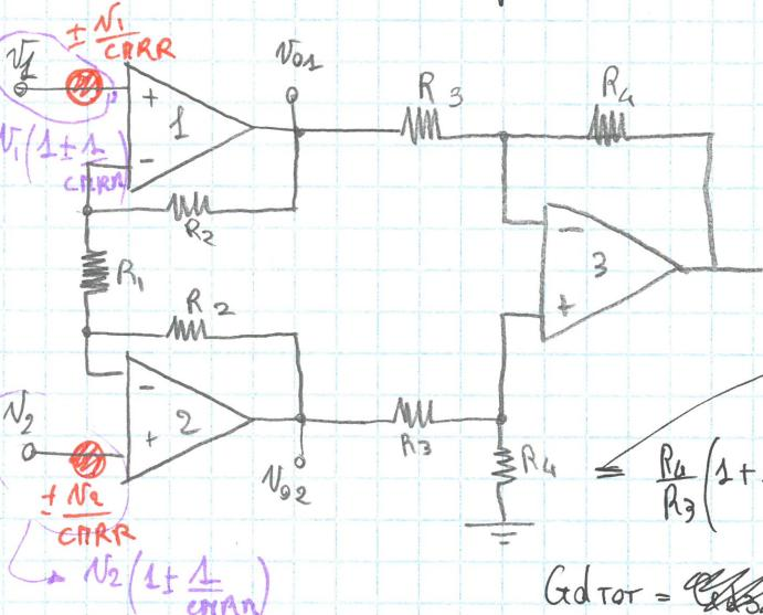
$$V_{out} = \left[ N_2 \pm \frac{N_3}{CMRR} - N_1 \mp \frac{N_1}{CMRR} \right] \frac{R_1 + 2R_2}{R_1} \cdot \frac{R_4}{R_3}$$
